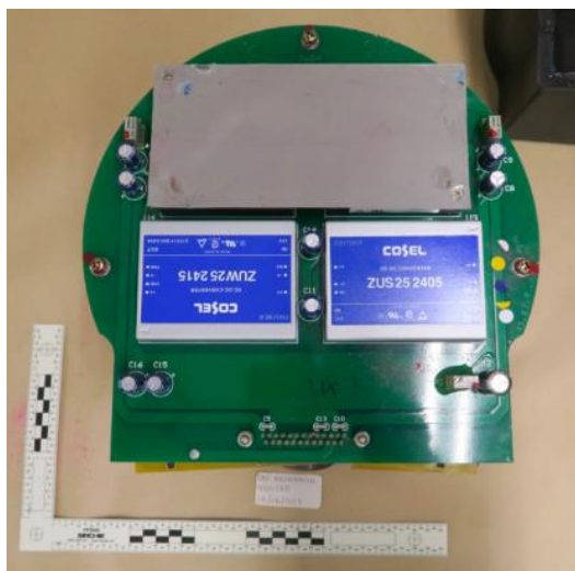
Serial number on the DC-DC converter: “ZUW25_2415” and “ZUS25_2405”
