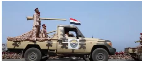
Figure 65.10. Mounted with 106mm recoilless gun similar to M40 or a variant of it
