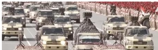
Figure 65.17. Mounted with 122mm MLRS with six tubes
