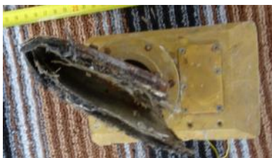
Figure 51.16. Part of one of the three actuator systems and control surface connector (top view)
