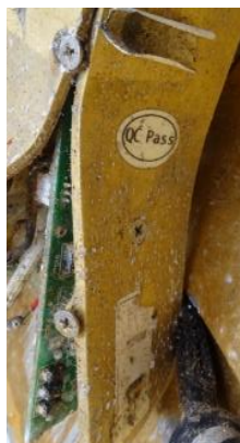
Figure 51.62. Part of one of the three actuator systems (side view) with “QC Pass” sticker
