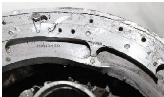
Figure 51.51. Jet engine part of a cruise missile used in the Houthi attack in September 2019 on ARAMCO installations in the KSA. Serial number in the format “100XXXXX” (100 followed by five digits)
