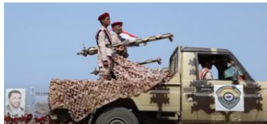
Figure 65.7. Mounted with 82mm recoilless gun similar to B10 or a variant of it
