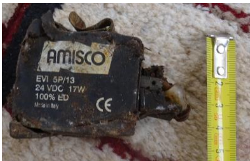
Figures 51.52. (up) and 51.53. (down) AMISCO solenoid coil (part of jet engine ignition system) 180
