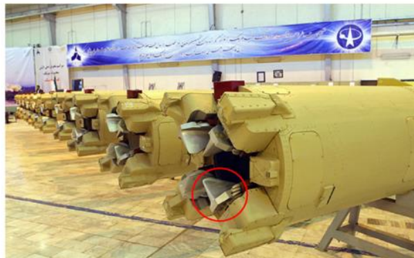
Figures 35.2. (up) and 35.3. (down) Jet vanes of Qiam ballistic missile manufactured in Iran
