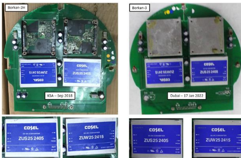
Serial number on the DC-DC converters: “ZUS25_2405” and “ZUW25_2415”
