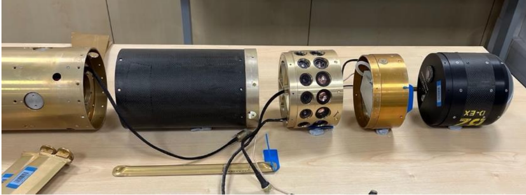
Figure 18.12 Seeker, air data computer, fuse and warhead of the “358” surface-to-air missile
