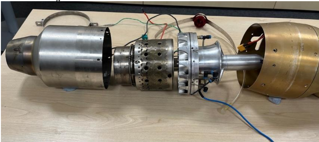
Figure 18.10 Gas-turbine engine of the "358" surface-to-air missile
