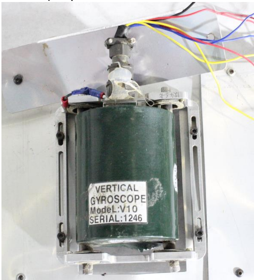
Figure 5.20 Model V10 Gyroscope from one of the “Sammad” UAVs used in the attack on 2 February 2022
