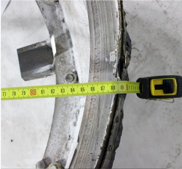
Figure 5.3 Detail showing the diameter of the missile (88 centimetres)
