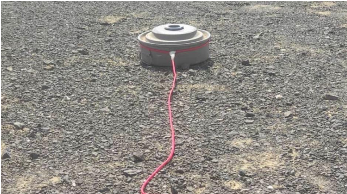
Figure 17.3 Explosive opening of the anti-vehicle landmine selected for sampling using detonation cord
