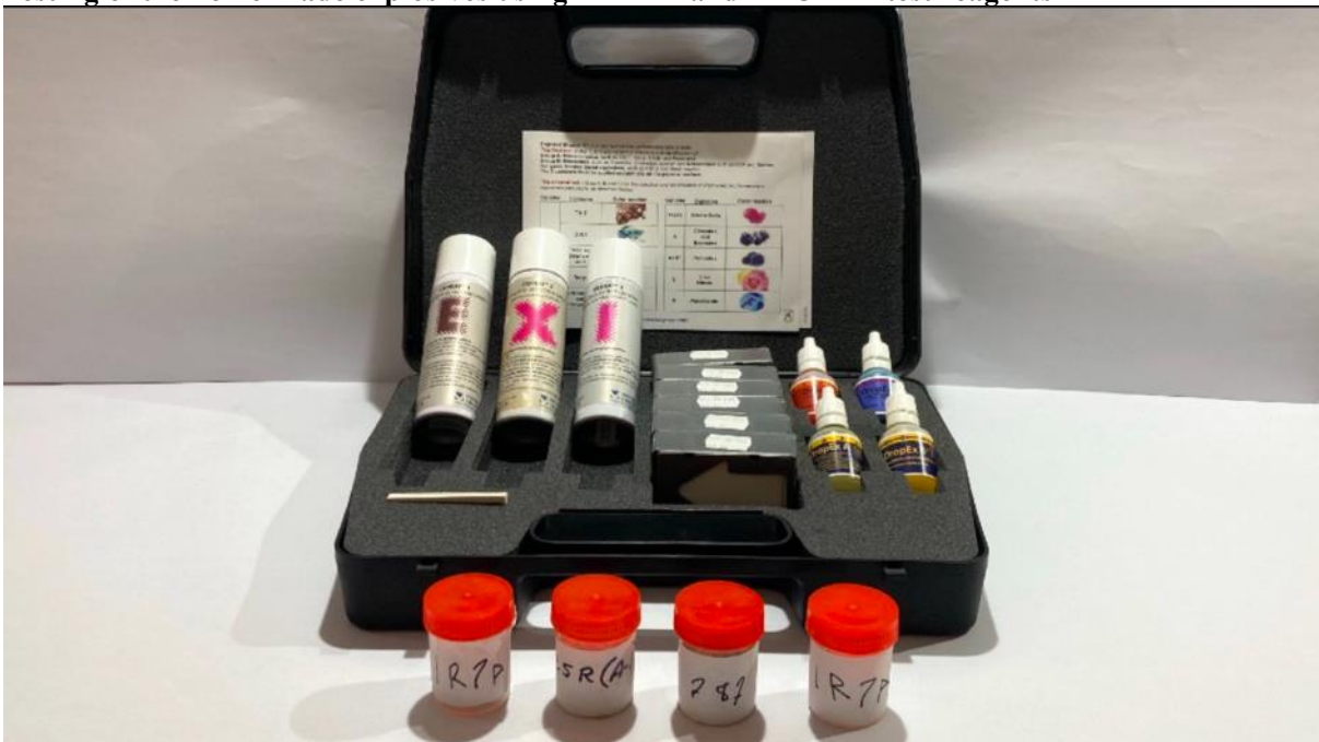
Figure 17.5 Testing of the home-made explosives using EXRAY and DROPEX test reagents
