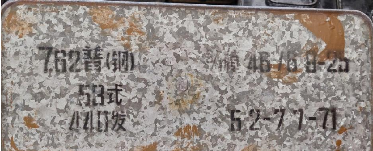
Figure 11.12 Markings on ammunition box indicating manufacture at State Factory 71
