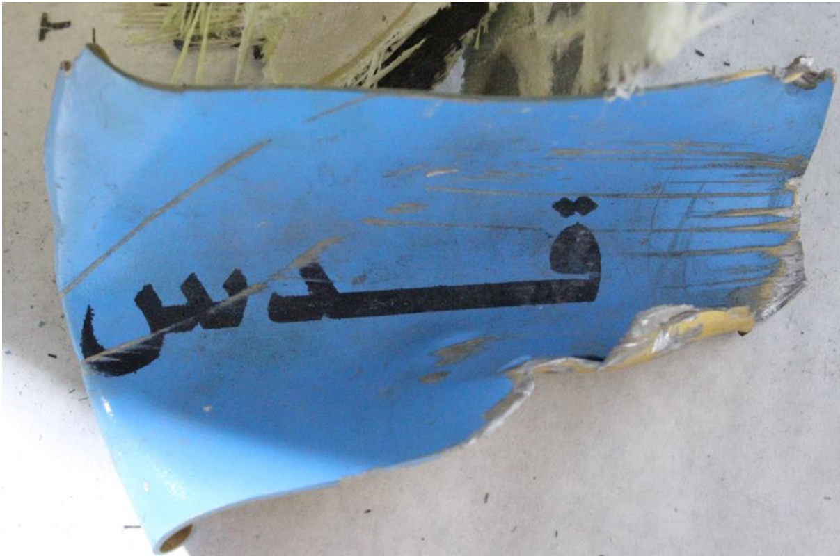
Figure 5.14 “Quds” marking on the debris of one of the cruise missiles
